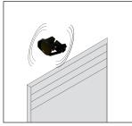
The sensor shall be firmly fixed to avoid any false activation by shocks or vibrations. It should not be mounted to high vibration surfaces such as a door canopy that houses the operating mechanism.
