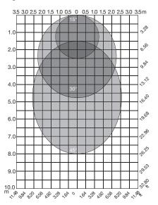
Mounting height: 7m with 3 different inclination angles.
