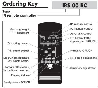
Note: For optimum results point the remote control at the sensor before pressing its buttons.
