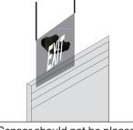
Sensor should not be placed near metal halide lights or placed behind any kind of protection layer or plate.
